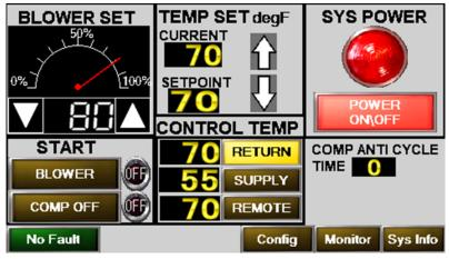
HMI MAIN screen - Control system functions.
